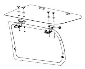
With the struts attached, close the panel carefully, again watching if it fouls as it closes. Once closed note any required adjustments to the door panel to align it with the car.
