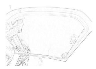
Once the weather seal has been glued into place, close the door panel and check the depth to ensure it aligns with the car and compresses the rubbers seal. If adjustment is required detach the gas struts and then loosen the hinges from the top supports, apply pressure evenly to the outside of the door where the hinge meets the door and re-tighten the bolts.
