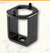
Roadsafe have available both the 'pin style' and '54mm' Hub Sockets to suit for Nissan Patrol. Hub Nuts in the early GQ's are a standard 'normal' hexagonal nut. Hub Nuts in the late GQ's (Series 2-on) & GU are circular with holes that require pins to slot in and turn. The Roadsafe 4H501 Hub Socket has prongs that slot into the corresponding holes. Roadsafe Hub Sockets are designed for use with a ½" drive, so you can use your standard socket set so tighten or remove the wheel bearings.
