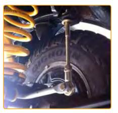
STB8828ET + STB8833ET - CUT TO DESIRED LENGTH TO SUIT FOR 2 TO 8" LIFT. STBEXTOO2 WILL NOT SUIT 100 SERIES WITH REAR BRACKET 48826-60010
