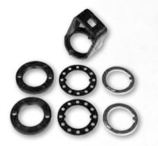
Roadsafe offer a kit that allows you to upgrade the GQ to the more advanced wheel bearing locking nut system as included standard on the GU. When changing or adjusting wheel bearings, jack the vehicle off the ground, remove the hub & nut assembly. Replace or repack the bearings, place the tab washer in, then thread the large hub nut on the stub. If you have installed new bearings, rotate the wheel when tightening – use your manual to get
