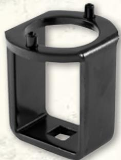
Roadsafe have available both the 'pin style' and '54mm' Hub Sockets to suit for Nissan Patrol. Hub Nuts in the early GQ's are a standard 'normal' hexagonal nut. Hub Nuts in the late GQ's (Series 2-on) & GU are circular with holes that require pins to slot in and turn. The Roadsafe 4H501 Hub Socket has prongs that slot into the corresponding holes. Roadsafe Hub Sockets are designed for use with a 1/2" drive, so you can use your standard socket set so tighten or remove the wheel bearings.
