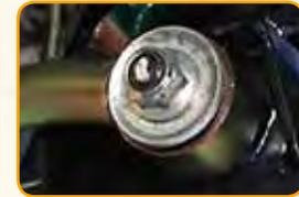
Note for Patrol Panhards. Where the Panhard is secured using a cupped washer on the Diff Mount - please ensure the washer faces outwards (so it 'cups' away from the diff). Do not have the 'cup' facing inwards.
