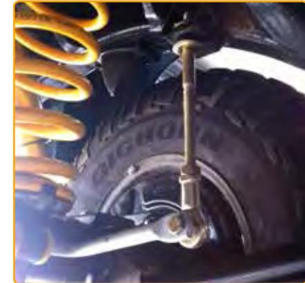
*STB8828ET & STB8833ET - CUT TO DESIRED LENGTH TO SUIT FOR 2 TO 8" LIFT. STBEXT002 WILL NOT SUIT 100 SERIES WITH REAR BRACKET 48826-60010*
