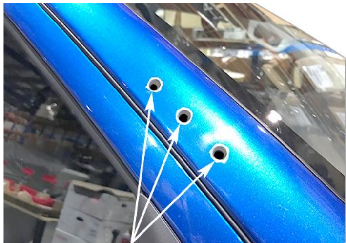
Drill A-Pillar Panel 8mm, Inner Panel 6.5mm
